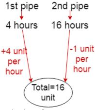
Rate of filling the tank by 1st pipe= 4 unit per hour Rate of emptying the tank by 2nd pipe= 1 unit per hour Net rate of filling the tank=4-1=3unit so required time=16/3=5  $^{1}/3$  hours Ans.
