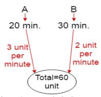
Rate of Filling the tank by A and B in 1 minute=3+2=5 unit So, total time taken by Pipe (A+B)=60/5
