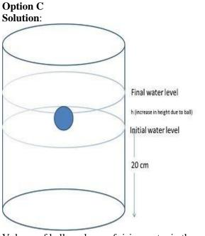
Volume of ball= volume of rising water in the cylinder  $4/3 * \pi^* r^2 = \pi^* r^2 * h$ 4/3\*6\*6\*6=4\*4\*hh=18 cm
