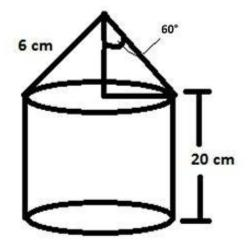
$sin 60 = P/H=r/6=\sqrt{3}/2$ => r=3\sqrt{3} cm In the cone; 6<sup>2</sup> = h<sup>2</sup> + r<sup>2</sup> h=3 cm Volume of Gunpowder= Volume of Cone+ Volume of Cylinder=1/3 \pi r<sup>2</sup>h + \pi r<sup>2</sup>h = \pi r<sup>2</sup>(1/3 h+h) =22/7\*27\*21=1782
