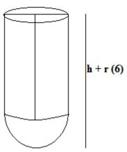
Volume of the container = Volume of the cylinder + Volume of the hemisphere Volume of the container =  $\pi 6^{2}h + (2/3) \pi 6^{3} = 576\pi$ =  $\pi 36 (h + 4) = 576\pi$ Solving we get h = 12 So the height of the container = 12 + 6 = 18 m
